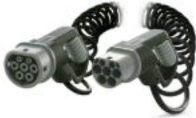
Charging cable, Connector, Plug, Charging cable with plug, IEC 62196-2 (type 2), Length: 4 m, Color of outer sheath: black, Number of phases: 3, Charging mode: Mode 3
