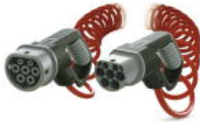
Charging cable, Connector, Plug, Charging cable with plug, IEC 62196-2 (type 2), Length: 4 m, Color of outer sheath: red, Number of phases: 1, Charging mode: Mode 3
